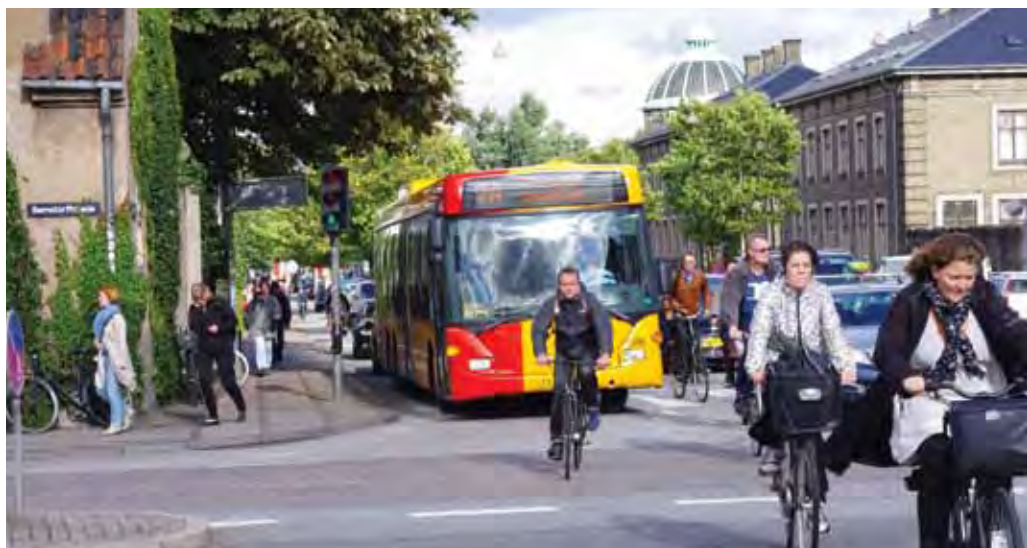
Shortened cycle track. Cars and cycles merge, which makes vulnerable cyclists in particular feel insecure. Tietgensgade, Copenhagen.
