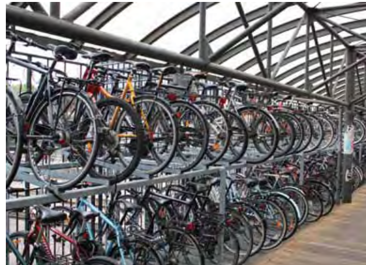
Capacity was doubled at the Aarhus railway station by replacing 500 ordinary perpendicular, front wheel spaces with 1000 two-tier spaces.
