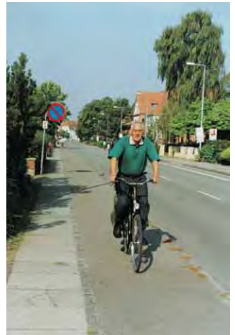
A separated, shared-use path can work when there are few cyclists and pedestrians.
