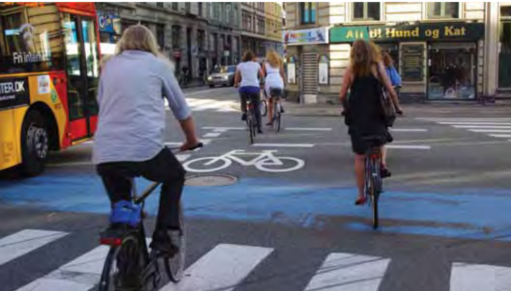
Blue cycle crossing, and international cycle crossing of the “one quarter type” indicated by a white dashed line on the cyclists’ left. Enghavevej/Vesterbrogade, Copenhagen.
