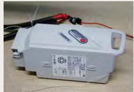
SAFE The BMS (Battery Management System) switches off quickly. In the second phase the electronics are bypassed. So the battery heats internally to over 100° C, but then cools again. Some fluid electrolyte has appeared, but no gases or other fluids.
