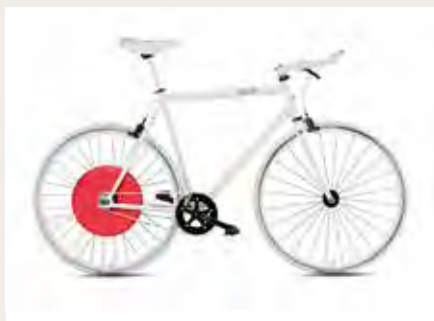
Copenhagen Wheel Pedelec 25 for retro-fitting. The drive is not the main focus, rather the gathering of sensor data on air quality and networking to data centres and other users.
