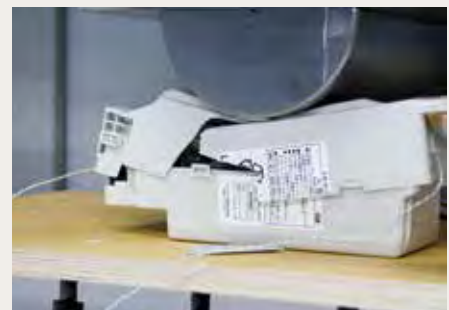
SAFE Mechanical destruction of the battery housing, squashing the cells but no heating, no leakage of gases or fluids.
