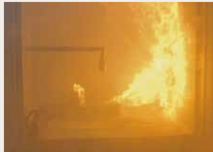
UNSAFE Eruptive conflagration shortly after exceeding the final charge voltage
