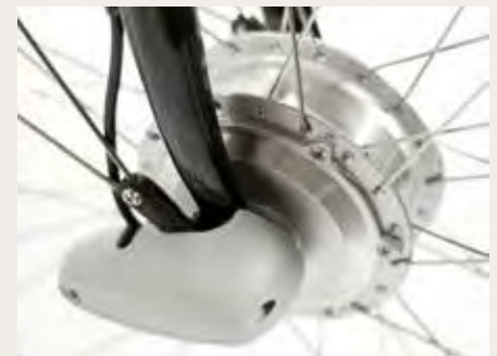
The best selling pedelecs 25 drive system in Europe in 2011 – the geared hub motor from the 8Fun company in China
