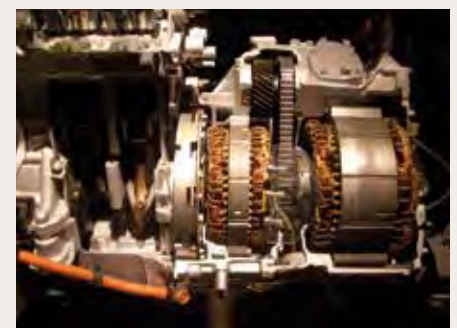
A role model for the pedelec – the principle of combining electric motor and IC engine, as solved in the Toyota Prius . For pedelecs it would work similarly, with the combination of electric and muscle power, for example in the futuristic prototypes from the company Nexxtdrive .
