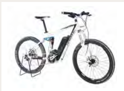
Haibike EQ Xduro Pedelec 25. Full suspension mountain bike, built around the pre-configured electrical components from Bosch .
