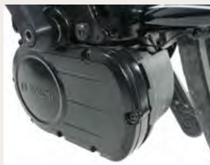
The crank drive motor from Bosch follows its successful predecessors from Japan, from Panasonic and Yamaha .
