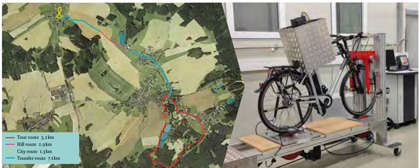
LEFT The three real world ExtraEnergy test routes: tour, hill and city. This is where since 2009 the test riders have been loaded with measurement sensors hand and foot – and the result is the digital test rider. RIGHT Here the digital test rider sits on the digital roadway which can precisely simulate the three test routes in Tanna: tour, hills and city. This lets anyone worldwide perform comparison test rides at any time and whatever the weather, and to compare the data with a vast archive of measured values.
