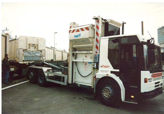
Figure 8: Transhipment of the container from truck to rail with ACTS system
